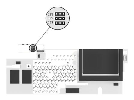
Figure 5-52. Display Configuration Jumpers
